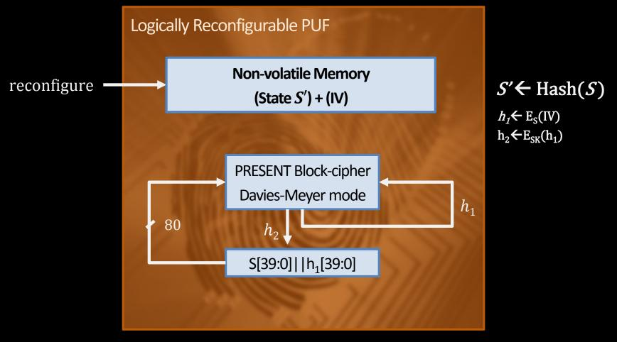
*IV* : Initialization vector – 64-bit  $h_1$  : hash-1 – 64-bit  $h_2$  : hash-2 – 64-bit System System System Security Lab Fraunhofer Security Lab Fraunhofer Security Lab Security Lab
