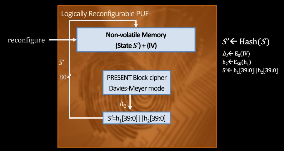
*IV* : Initialization vector – 64-bit  $h_1$  : hash-1 – 64-bit  $h_2$  : hash-2 – 64-bit System System System System System System System System Security Lab System System
